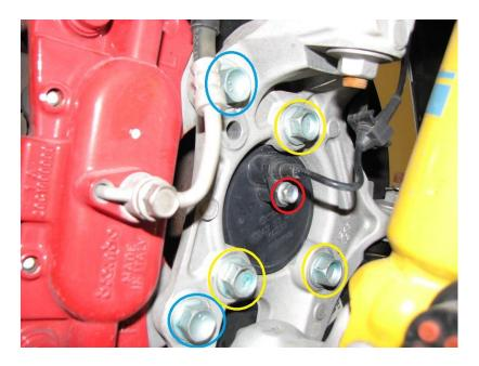
**2.7.** The hub can then be removed from the car, along with the OEM backing plate which we will be replacing.
