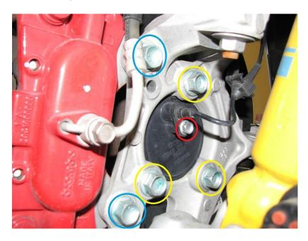
**2.5.** With the caliper loosened, you can rest it on the LCA. Remove the rotor from the vehicle.
