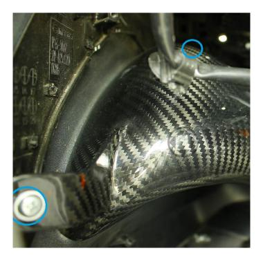
**3.7.** The fog light should be fully installed at this point and not hitting anything on the car. Repeat the same steps on the other side of the vehicle.
