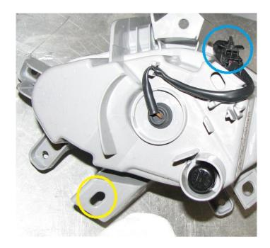
**3.5.** Remove the wire junction connected (circled in red below) and move it from the front of the bracket on car, to the rear of the bracket (as shown).
