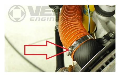
**5.6.** With this duct routing, we found it best to use (1) zip tie to hold the hose near the front of the LCA. This is circled in blue below. **Ensure that the hose will not rub on anything sharp or the hose can be damaged.**
