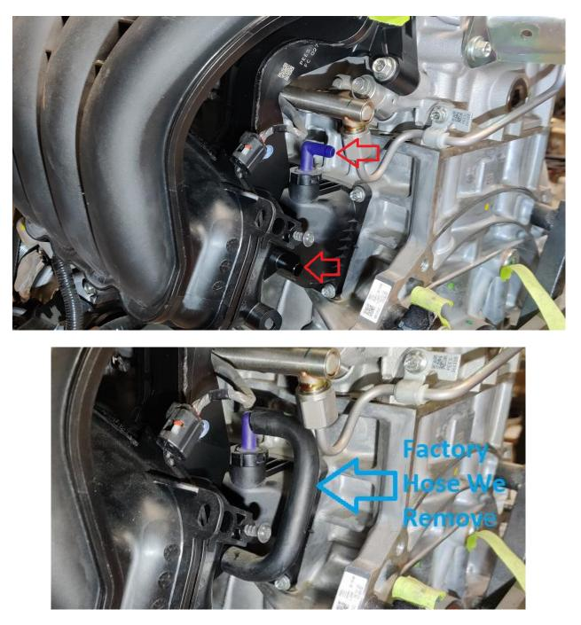
**2.8.** We do \*not\* recommend removing the intake manifold; as it is a chore to do so. We did on our install to inspect how much blow by we were getting but it was a lot of work to get it fully out. You will have to use your hands and reach below in this area to find a "U-Shaped" hose which connects the intake manifold and the block. **Remove this hose.** The block hose location can rotate, so feel around for this and if the hose location rotates, you found the block PCV hose location.
