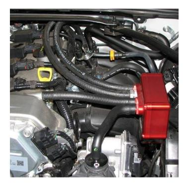
**2.15.** The single most important hose location is the hose going to the PCV value on the AOS. This \*needs\* to go to the hose that attaches to the intake manifold for proper operation.
