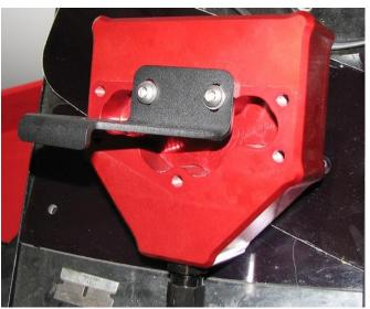
2.13. We can now install the AOS onto the bracket shown below. Utilize the fender washer and a 16mm long BHCS to fasten this to the car.
