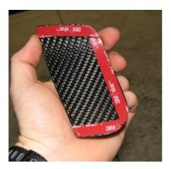
**2.12.** We can now install these covers as shown below. Firmly press these into the wing to get proper adhesion.
