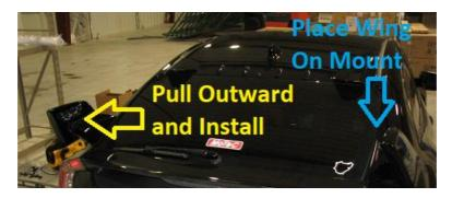
**2.7.** Install supplied M6 bolts and washers into the rear wing as shown below. Loosely install all (4) bolts before tightening.
