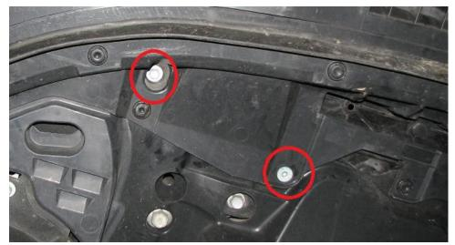
**2.8.** The remainder of what is holding the underbody panel on should be plastic rivets. These are removed by popping up the center section and then pulling the unit out. Most of these are circled below in yellow, there are a few others towards the back of the panel that needed removed as well.
