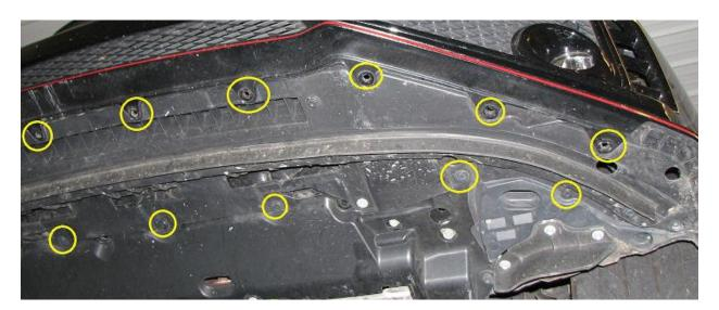
**2.9.** With all the fasteners removed, we can remove the panel by pulling it down and out from the bumper. You can now see all the plastic rivets removed and what all removes from the car.
