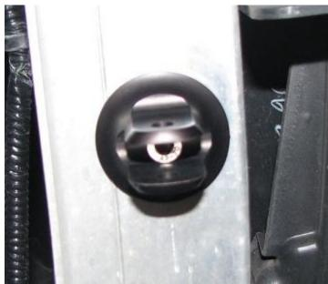
**3.10.** Before fully tightening the clevis, we will want to snake a support rod through the grill to ensure it lines up well with the clevis. The goal is to have the support rod going longitudinally with the vehicle.
