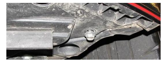
**2.6.** Remove the Philips screw on the back of the front lip, as shown below.
