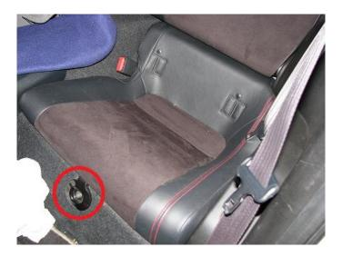
**2.4.** The rear of the seat needs pushed down and then forward to unlatch from the chassis. The seat has a loop that attaches to the chassis, it is located roughly in the middle of the seat. Shown below is the bottom of the seat cushion when removed.
