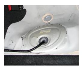
**2.6.** Use a screwdriver to pull up on the metal lid. With a razor, cut the black silicone to aid in removal.
