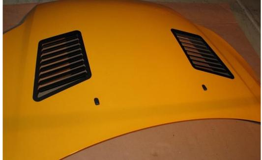
**2.29.** The wickers are installed from the bottom side of the hood louver. These increase evacuation of under hood pressure and temperature. (Note: Below picture is an FRS/BRZ install.)
