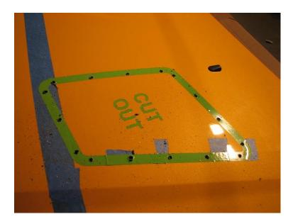
**2.18.** Enlarge the inside holes to 1/4" or 3/8" as shown below. Enlarge the 16 mounting holes to 1/4" initially.
