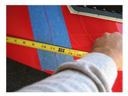
2.9. Do this to both sides and lay a piece of painter's tape across the whole hood keeping it as lateral as possible. NOTE: Yellow car is 2011-2014 MY install, Red car is 2015+ install. Disregard template placement at this time.
