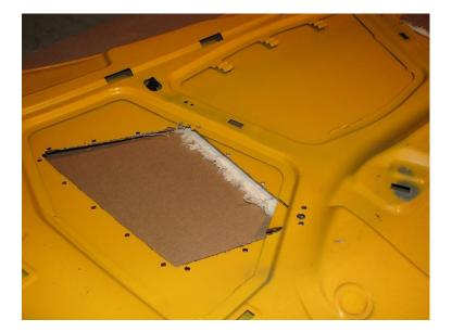
**2.22.** On the bottom side of the hood, you'll see the mounting holes through the structural metal. We'll use these holes as guides for cutting of the structural sheet metal. These few holes are circled in red below.
