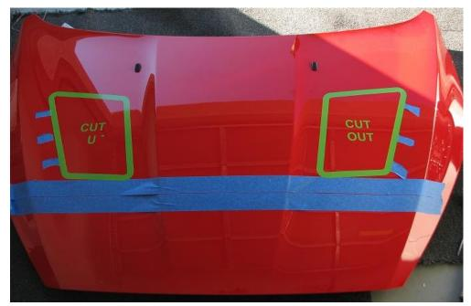
**2.16.** For the remainder of the install, the different model years do not deviate so we will be showing pictures of the 2011-2014 MY Focus ST only. Using the center punch (or a sharp unused tap) and hammer, gently center punch all 16 holes per side. The holes are located with crosshatch markings, center punch the intersection of each. Also center punch the inside (4) corners of the template.
