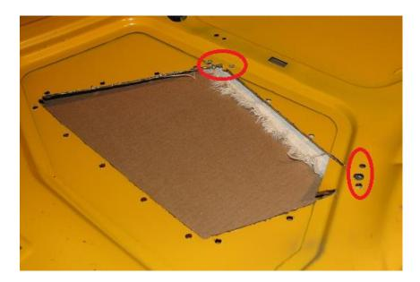
2.23. Using the cutoff wheel again, remove all of this material while giving ample room to tighten the nut on. This is shown below. \*Be sure that you do not cut through the hood's skin.\* This is likely the most difficult portion of the entire install!
