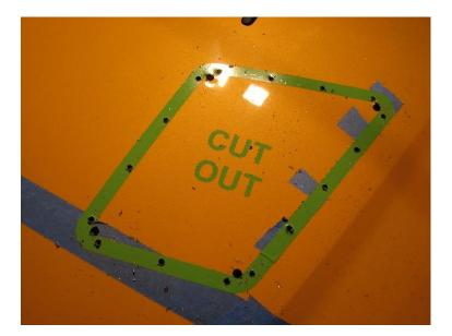
**2.19.** Using the template as a guide, cut out the section marked "cut out". The hood is steel and the paint is very easily burnt! This is normal and will be covered up with the flange of our hood louver.
