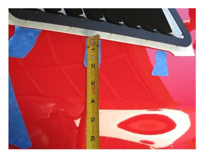
**2.13.** Ensure that all tape edges laid are equal side to side.
