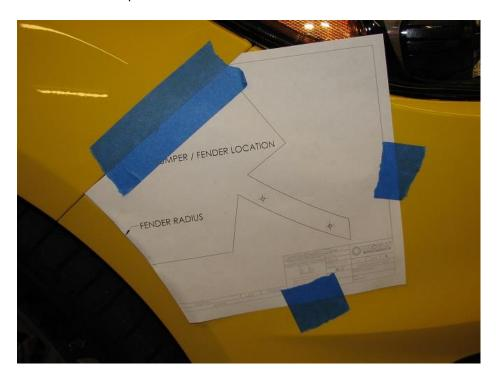
**2.8.** Before marking the holes with a center punch or tap, ensure these holes on the template line up with the dive plane's holes and that the dive plane mount surface fits with the bumper well.
