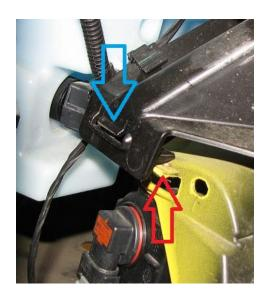
**2.16.** With the nuts and washers on the rear side of the bumper, you can tighten the bolts on the dive planes. We found tightening the bolts from the outside while holding the nuts on the rear with a wrench easiest.
