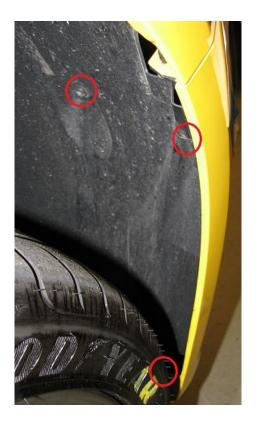
**2.5.** To further improve ease of install, you can loosen the bumper by removing the single plastic push pin with a flat head and pulling the bumper away from the car.
