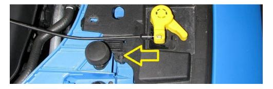
**2.8.** Remove the headlights from the vehicle by removing the two bolts holding it in. These are circled in red below, but the headlight is already removed.
