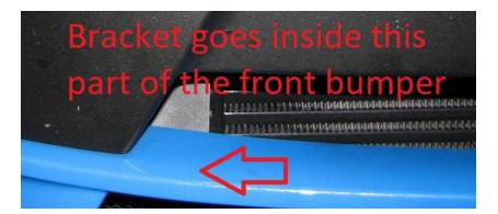
**2.21.** Loosely re-install the front bumper as we will begin making a few holes in the front bumper. Estimate the location of the rivet-nut on the bracket. Using a bolt in the bracket, you can use the bolt head to estimate the location of the rivet nut by feeling for the head of the bolt through the bumper.
