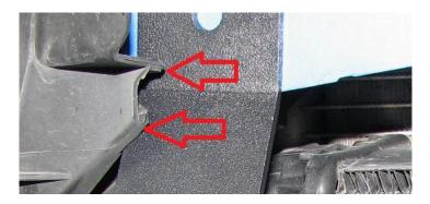
**2.19.** Below is the driver side showing the plastic being trimmed.
