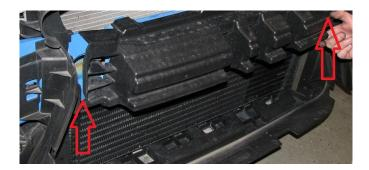
**2.16.** Below is an image of where the bracket will sit with the bumper installed. You will just barely see the brackets when installed.
