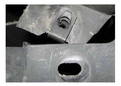
**2.31.** Reinstall the torx bit on the front of the fender liner (in front of the front wheel).
