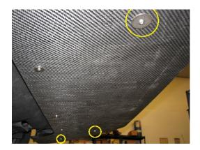
**2.36.** Loosely install the rear (3) bolts and washers. These are the M5 x 60mm Long BHCS. On the top side of the splitter, we will want to install (2) of the nylon spacers on each bolt location.
