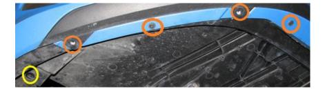
**2.11.** Near the front of the front tire, there is a bolt on the bottom of the front bumper. This is circled below, and above, in yellow and should be a torx.
