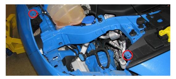
**2.9.** With the front of the car off the ground, we will want to start by removing the underbody plastic vertical piece. You remove this by unscrewing the (3) bolts circled in red below. This will be removed and left off.
