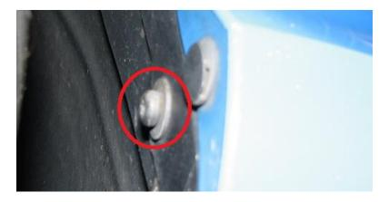
**2.28.** From below, pull the fender liner rearward to expose the factory clip-on nut.
