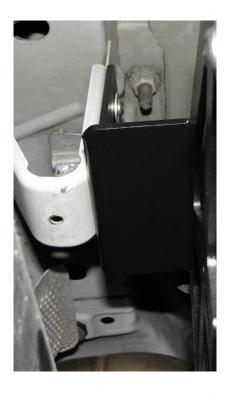
**2.6.** Moving to the rear brackets, we will start with the driver's side (non-exhaust side) rear bracket. This bracket has (3) holes on the bottom flange, which is shown below. The flange points to the rear of the vehicle when it is installed. Use (2) 16mm long bolts, washers, and nuts to install the bracket.
