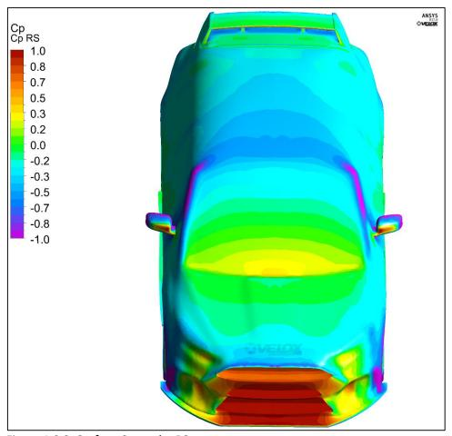
Figure 1.3.3: Surface Cp on the RS
