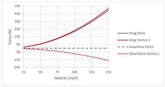
Figure 1.2.1: Aerodynamic Forces at Speed
