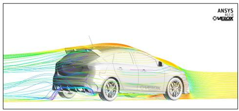
Figure 1.3.2: Streamlines from Rear Diffuser
