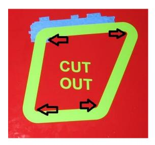
**2.12.** Using the smallest drill bit, 1/8", drill through the multiple layers of the hood as shown below. Use high speed and light pressure to not break the bit or go plummeting through the hood and scratching it.
