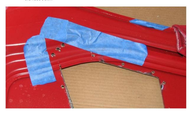
**2.18.** Using the cutoff wheel again, remove all of this material as well. This is shown below. \*Be sure that you do not cut through the hood's skin.\*
