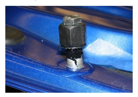
**2.10.** Utilize the 9/16<sup>th</sup> wrench to hold the nut and a 10mm socket, tighten he rivet nut into the hole. A fully installed rivet nut is shown below. The slight excess of sealant is desired to reduce rusting.
