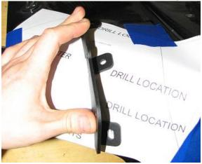
2.15. Using a center punch, mark the (3) holes per side for drilling.
