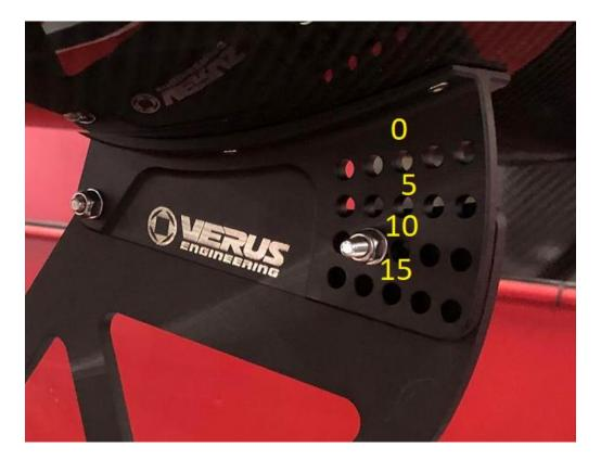
**2.28.** To finish installing the rear wing, we have to install the endplates. We offer both carbon (upgrade) and sheet aluminum (standard). Both install the same. We include aluminum washers for M4 FHCS, and o-rings to reduce marring of the aluminum of carbon fiber. Install the o-ring on the washer, and install into the endplate and rear wing as shown below. Finger tight should be plenty.
