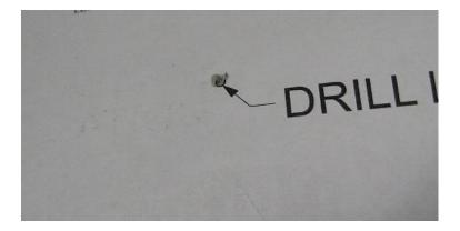
2.17. There are two ways to install the trunk mount to the trunk skin; bolt and nut or with rivet nuts. The choice is yours. If you are using rivet nuts, open these holes to 3/8". If you are using bolts and nuts, open the hole sizes to 9/32".
