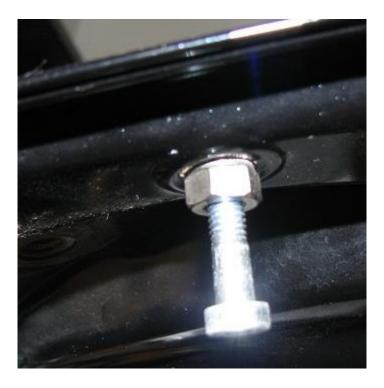
**2.32.** Then, while slowly closing the trunk, watch the SHCS and see how close it comes to touching the trunk hinge mount (shown below). You will want the SHCS to hit this piece on the hinge location when fully closed to reduce the amount of movement on the trunk at speed.
