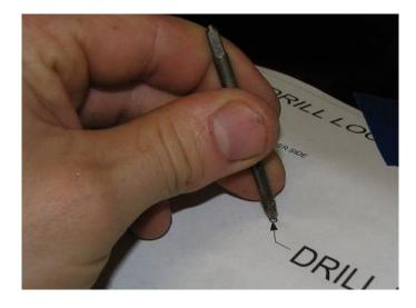
**2.16.** Using a starter drill bit, drill the (6) holes. An 1/8" drill bit works well for this.
