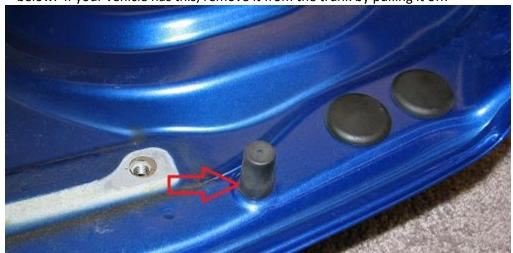
2.8. We need to open this hole to 3/8" to install the rivet nut. If you did not have a rubber bumper in this place, you will need to drill a new hole. Ensure you do not puncture or go through the bottom side too quickly. You can cause the skin's sheet metal to deform if the drill bit hits it.
