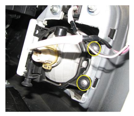
2.25. We used electrical tape on the fog light plug to do our best at keeping the water out of the connector for possible future use.
