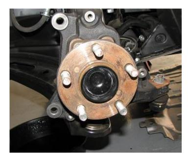
2.10. Loosely install the new Velox Motorsport backing plate on the knuckle. Place the hard anodized spacers behind the backing plate. The wheel speed sensor should remain installed and will be placed between the knuckle and the carbon duct.
