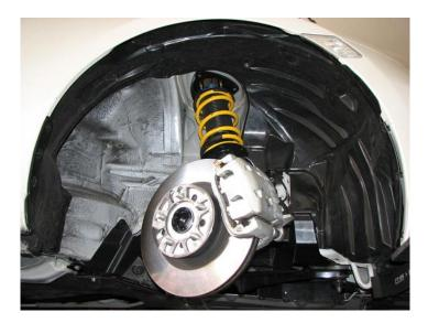
2.21. Due to the splitter and front wheel deflectors, we opted to remove it from the rear and fold it forward. The fender liner is removed with various styles of plastic rivets and push pins, using your best judgement and the plastic removal tool, remove these.
