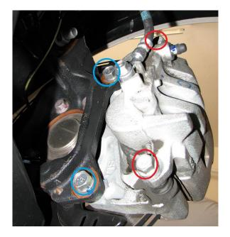
2.7. Then remove the brake pad bracket by unbolting the 17mm bolts (circled in blue above). Below is what it will look like with both bracket and caliper removed.
