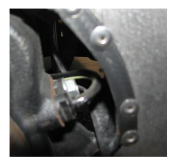
2.12. Using your mark as a guideline and one of the two strips of foam, wrap the wire to protect it against damage.
