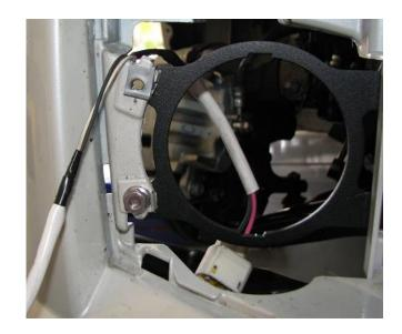
2.31. Slide the fog light duct into the bracket paying attention to the locating tabs (the duct should exit towards the middle of the car). Shown below is the duct installed into the bracket.
