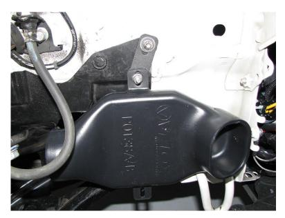
2.39. With the duct installed, we can better judge how the relief cut needs to change. Below is where we finalized the cutting of the duct at.
