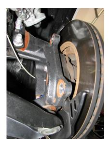
2.8. Remove the rotor. Dependent on how long the car has sat, if it sees snow/salt, the rotor may need to be forcibly removed. You can do this with a rubber mallet or the bolt holes on the rotor surface. Below is a photo of the rotor removed.
