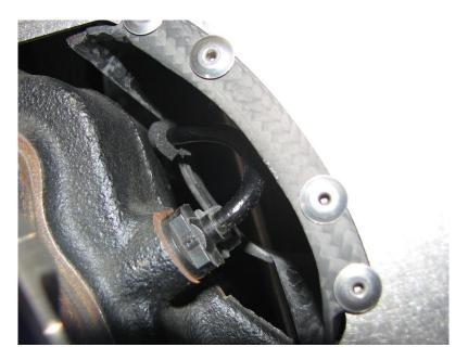
2.14. Fully tighten the (3) 5mm hex flanged BHCS.
