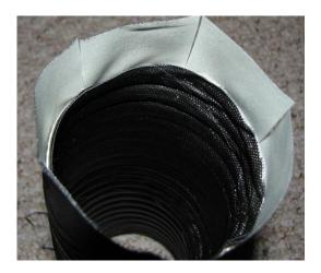
2.42. Fold over each slit pressing firmly against the hose.
