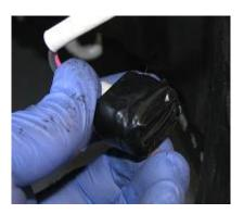
2.26. Place the fog light bracket around the duct and then the duct/bracket assembly into the hole where the fog light used to reside. Using the OEM screws, tighten the bracket down. The plastic fog light should have a little play but not a lot.
