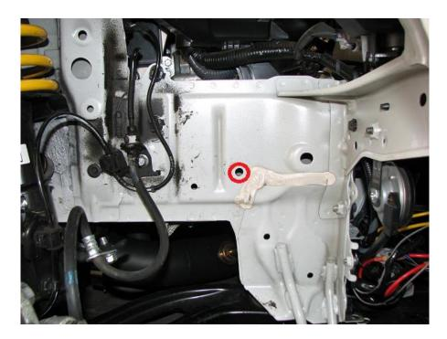
2.34. We recommend using a shop vac and trying to suck out all metal filling before they drop into the frame. We also recommend painting this hole or using sealant when installing the rivet nut to reduce the chances of rust.
