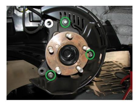
2.9. Remove the OEM backing plate by unbolting the (3) 12mm bolts circled in green above. Below is a photo with the backing plate removed.
