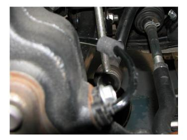
2.13. Re-install the backing plate with the supplied hardware and position the wire so that it is safely and nicely squeezed between the knuckle and the duct. The goal here is to have no movement and a snug fit to ensure the wire does not get abraded over time.
