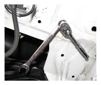
2.36. You will feel it get significantly harder to tighten, this is a sign the rivet nut is fully installed. Below is a picture of a properly installed rivet nut of this style.
