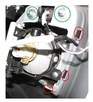
2.30. With the bezel removed, we can install the fog light bracket with the supplied M5 BHCS and serrated nut hardware. In the below picture, you can see the OEM clip on the top, and the supplied hardware loosely installed on the bottom. We recommend using OEM clips if your car has them, but those without fog lights likely do not. Install an M5 bolt and washer on the back side, with the serrated nut on the front and tighten.
