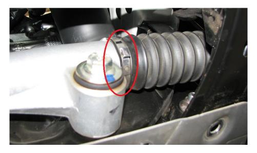
2.56. Once the strap is removed, pull the boot off towards the outside of the car, and slip one or more of the steering rack limits onto the rack. The open end should face forward as shown below.
