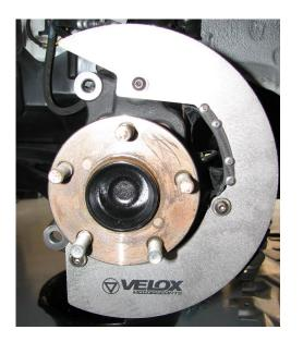
2.11. As you can see below, the wheel speed sensor wire is slightly rubbing on the carbon duct and the knuckle. Mark this location and remove the backing plate.
