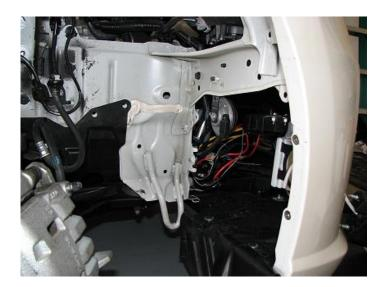
2.22. Remove the engine bay plastic piece by removing a few more plastic rivets from the inner fender and from the bottom of the car. This plastic shroud piece is circled below.
