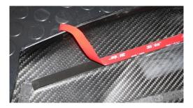
**2.12.** Place the spoiler on the car. Once happy with location, pull one tab at a time and press/massage the spoiler into the chassis. Repeat this with as many "pull tabs" as you created until the entire spoiler is installed.
