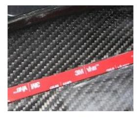
**2.10.** With the double sided tape installed on the spoiler, we can mark the outsides of the spoiler so that it is centered. We used painters tape to do this.
