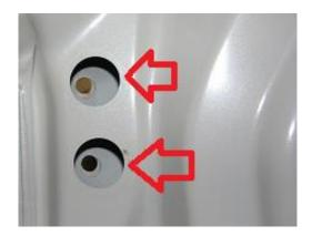
**2.3.** We can now remove the (4) bolts that hold the OE spoiler on the car. These are 8mm bolts.
