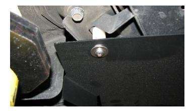
**2.20.** Finally, install the last M6x1.0 BHCS, washer, and nut as shown below. This will be going to the bracket we installed in step 2.13.
