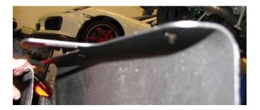
**2.9.** Remove the burr from both sides of the rear diffuser with a chamfer bit.
