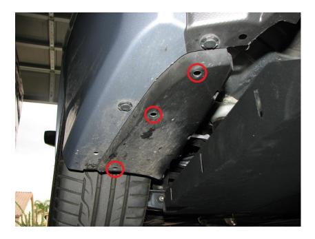
**6.9.** Using the supplied rivet nut installer and rivet nuts, install one of these in each of these holes. You will use a 9/16" wrench on the nut and the 5mm socket on the bolt. Tighten these until the rivet nut is fully installed. The serrated end of the rivet nut installer is used towards the rivet nut.
