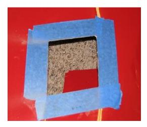
2.21. Once you have these cut out, you will want to test fit the louvers and find out where you need to shave off more to ensure un-obstructed. To shave off small amounts, we recommend using an abrasive wheel (shown below) on a 90 degree grinder.
