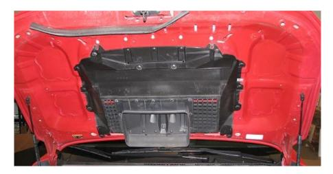
2.6. On the hood struts, utilize a small screwdriver to remove the clip, located with the arrow below. On the right side of the below image the clip is removed. This allows the strut to come off the hood when we fully remove the hood.
