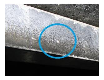
**3.10.** Using a starter drill bit or a pilot sized drill (1/8"), drill the center punched hole out. Using the 1/4" drill bit, increase the size of this hole to 1/4" as shown below.
