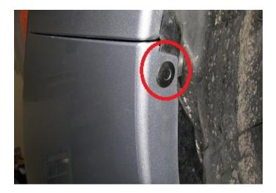
**3.4.** Moving to the top of the bumper, we need to remove the plastic rivets here as well, and the 10mm bolts scattered throughout. The 10mm are circled in yellow. The plastic rivets are circled in blue.
