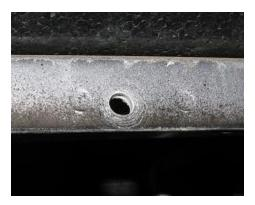
3.11. Using the tape measure, the hole to hole spacing should be 20.0" as shown below. Using the same procedure (center punch, pilot hole, 1/4" hole), drill this hole out as shown below as well. Once again note, the hole is drilled between the two spot welds (blue arrows), this is important as drilling through a spot weld is difficult.
