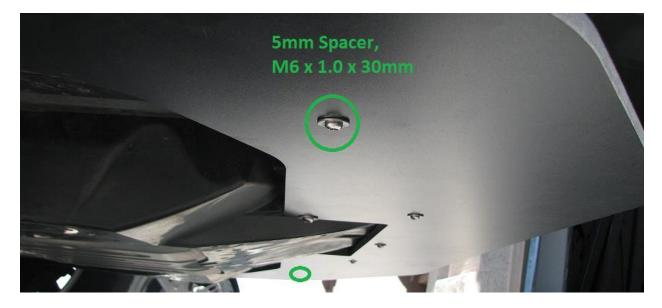
**2.20.** The front most three units (circled in yellow) receive the longer M6 x 1.0 bolts, which are 40mm in length. These three holes receive between 5 and 10mm of spacers typically. Use the extra provided washers to achieve thicknesses between 5 and 10 mm.
