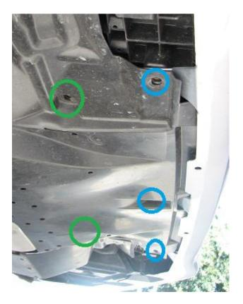
2.18. It's time to install the splitter now. You'll want to install all the bolts loosely first, by hand! The rear (4) bolts are M6 x 1.0 x 30mm long are installed without any spacers (circled in red). The rear two middle bolts are the M8 x 1.25 x 70mm long bolts, they need the 40mm nylon spacers installed between the splitter and the chassis (circled in blue).
