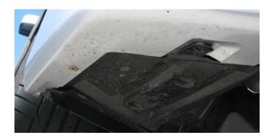
**2.14.** Below is a photo of the middle three rivet nuts installed on the car. Note how the rivet nuts are above the bumper tabs.
