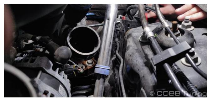
5. Slip the left side tube into the coupler and get it seated, but don't tighten the hose clamp yet. Make sure to seat it into the ball socket that holds it in place.
