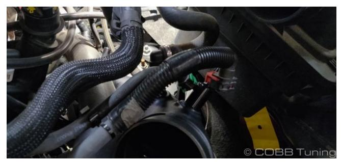
6. Install the factory breather lines and bypass valve recirculation tube, these are fairly straightforward as the sizes are different so it will only fit in one spot. Some of them may require turning the coupler or shifting some of the zip ties/tie downs that hold them together back along their length. Make sure they are loose and free to move, they use hard plastic in the end fittings and if they're tight they may break when stressed repeatedly while driving.
