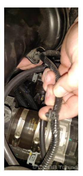
Disconnect the three vacuum connections on the left side inlet. Pay attention to how they come off, the red clip releases by getting squeezed inward while pulling out the tab, whereas the green one will go outward to release. The blue one will get squeezed and wiggle off.
