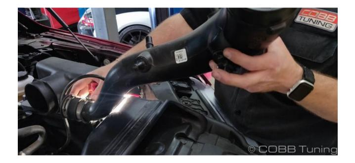
9. Swap over to the passenger's side wheel well, and remove the same inlet to turbo hose clamp you did on the driver's side.
