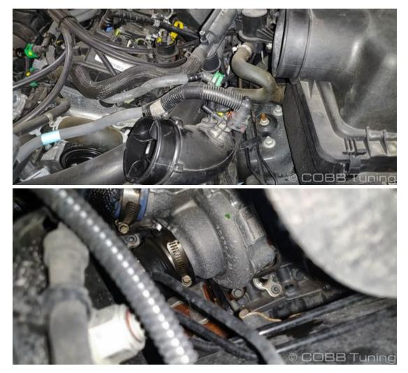
8. Partway down the inlet tube has a small ball pressed into a rubber socket, pop this out with your trim tool and remove the inlet tube from the car.
