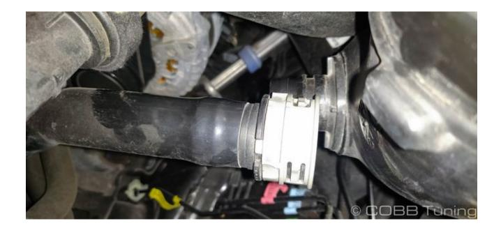
7. Looking into the driver's side wheel well, unscrew the factory hose clamp going from the inlet to the turbo using your 7mm.
