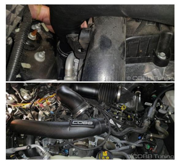
4. Moving over to the left side loosely install the coupler with the remaining medium hoseclamp before loosely placing the large hose clamp over the opposite end
