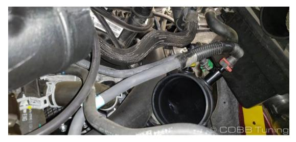
7. Install the central y-pipe onto the inlets and the airbox.
