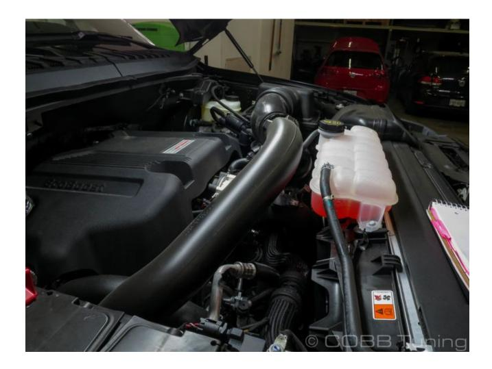
2. Once it's cooled down, Start by undoing the center intake "y-pipe" from the two turbo inlets and airbox using your 7mm nut driver.
