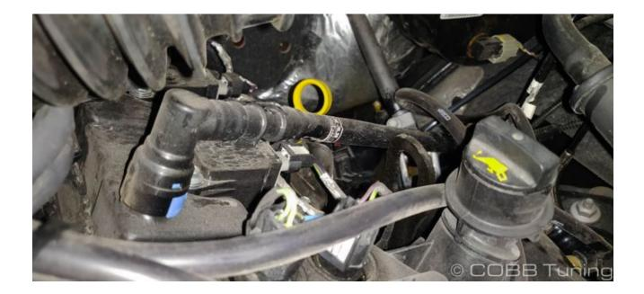
Disconnect the bpv hose from the intake and the BPV itself by turning left 1/4 turn. Sometimes it will be stuck due to dirt or debris getting into the clip. Softening it with some wd40 or water can make this more simple.
