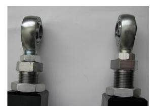
**6.8.** Once happy with the LCA set-up off car, it's time to put it on car. If you have the spherical rod end, place (2) of the bushings on either side of the rod end as shown below
