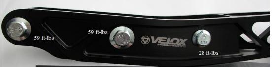
**6.12.** With the LCA fully installed, it is time to dial in camber back to OEM spec \*if that is what you wish to do\*. To do this, use a 1" wrench on the adjuster and thread it in and out till the measurement from left wheel to right wheel is the same as before install. Once satisfied, snug both lock nuts. The spherical/poly bushing is ¾" while the adjuster to LCA is 1.25".
