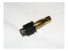
**2.8.** Place the rivet nut into the hole. If you'd like to use the rivet nut backing washer, you'll need access to the top side of the black plastic piece. The black plastic will go between the head of the rivet nut and the washer. Note, the backing washer is not necessary but will decrease the chance that the rivet gets pulled through, we did not use the washers personally.
