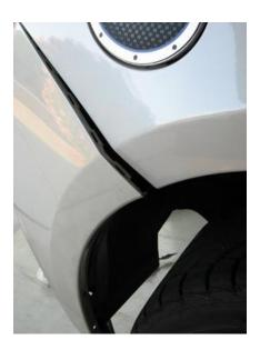
**2.6.** Moving back to the bottom side, pull the bumper outward and we gain access to the hard black plastic piece we will be installing the rivet nuts. The rivet nuts are installed in the picture below.
