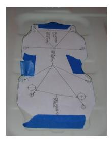
2.9. Using the center punch (or tap) and the hammer, we can center punch each of these holes. Ensure that the template does NOT move between each hit. Below is the picture after each hole has been center punched from the underside.
