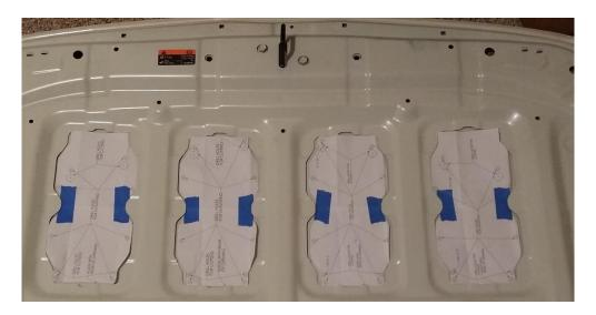
2.8. The templates should fit nicely in-between the structural sheet metal on the bottom. We started with the smaller side vent first, shown below.
