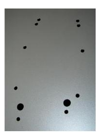
2.13. Clean each of these holes up from burrs with the countersink tool. Hit the top and bottom just briefly to break the edge.
