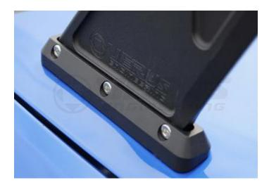
**2.31.** Reinstall the trunk onto the vehicle. Torque the 12mm bolts to 12-16 ft-lbs.
