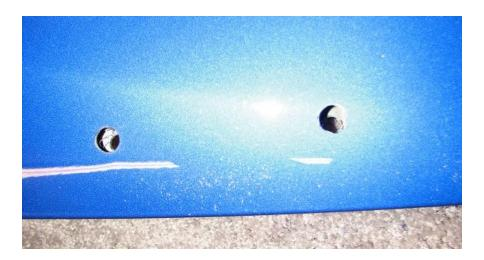
**2.18.** With the holes slightly larger, we can now use a carbide bit and grinder to open these holes up larger. You will want the holes to be slightly larger than bungs on the mount.
