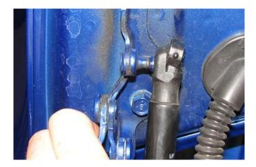
**2.4.** With these removed from the trunk points, we can remove the (4) 12mm bolts from the trunk and remove it from the vehicle. A second set of hands is definitely helpful.
