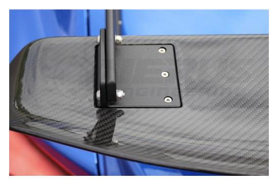
**2.33.** There are (5) AOA for the rear wing, 3, 6, 9, 12 and 15. Below is a photo showing how to choose each AOA with the rear adjustment location.
