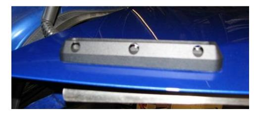
**2.30.** At this point, we can install the uprights into the trunk mount utilizing the (3) M5  $\times$  0.8 SHCS provided. Torque to 4 ft-lbs.
