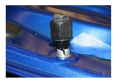
**2.15.** Utilizing the 9/16" wrench to hold the nut and a 10mm socket, tighten the rivet nut into this hole. A fully installed rivet-nut is shown below. The slight excess of sealant is desired to reduce rusting.
