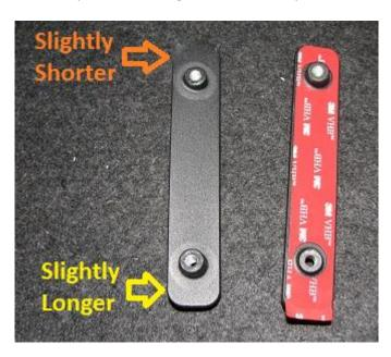
**2.23.** We now install the strengthening bracket on the bottom side of the trunk as shown below. Utilize the M6 x 1.0 Low Profile SHCS, with the jam nut install. Note the bracket orientation.
