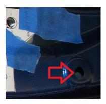
**2.14.** Once this hole is 3/8", we can install the supplied rivet nuts. We recommend a bit of sealant to help reduce the chance of any rust. This is shown below.
