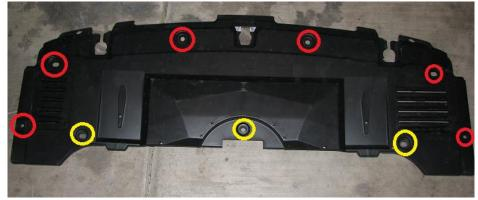
**2.5.** We now install the rivet nuts into the car's underbody. View the below photo to ensure the correct holes are used. *No holes should need to be drilled!* The photo below is only the passenger side of the car but the driver's side is a mirror image.
