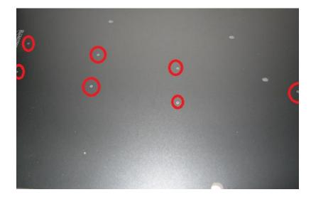
**3.3.** Utilizing the center punch and counter sink, increase the size of these engraved holes to decrease the chance of the drill bit wandering while drilling. Using a drill and 1/4" drill bit, drill the 16 holes as straight through as possible. Place the splitter on something soft to reduce scratching the surface (I used a towel on the leading lip and then propped it up on the wood as shown below).
