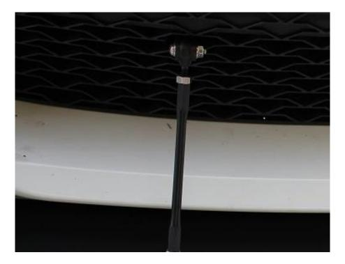
**3.16.** Using the 4mm allen wrench and the 10mm wrench, tighten the rod end into the clevis, a washer is used between the bolt and the clevis. Use the 25mm long bolt and the M6 flanged nut on the other side.
