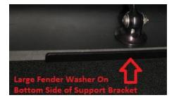
**3.21.** Ensure that the splitter is near horizontal by using a level. The front of the splitter's level is now controlled by the support rod system. Lengthen it to lower the front of the splitter, shorten it to raise the front of the splitter. **The splitter rod is both left hand and right hand thread, keep this in mind.**
