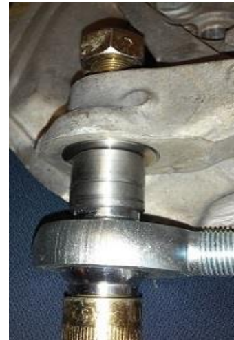
When tight, the conical spacer should be flush.
