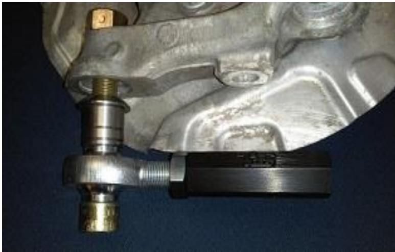
Make sure the conical spacer is in proper position.
