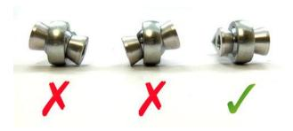
5. Once installed, ensure that both of the FK Rod Ends (2, 3) are centered and have full articulation. Lock them in place by tightening the Blue Titanium Socket Head Cap Screws (6) with a 3/16 allen wrench to 150 **IN. lbs.**
