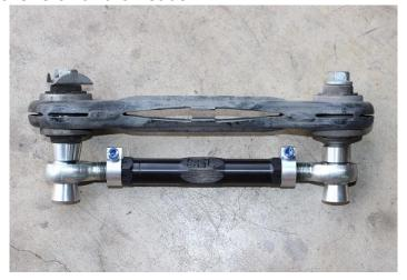
4. Install the SPL Parts Arm using the OEM hardware. Please ensure the Tapered Stainless Steel Spacer (7) provided mates up with the tapered section of the knuckle. Tighten the nuts to 73.7 **ft. lbs.** (100 N/M) at both ends. **DO NOT OVERTORQUE!** SPL Parts is not liable for any issues due to overtorque.
