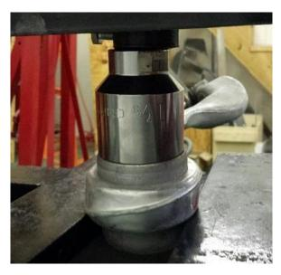
bore of the arm, and smooth any nicks or burrs. The same socket can then be used to drive in the new bushing. Again, make sure to align the driver and bushing to go in straight and not bind.
