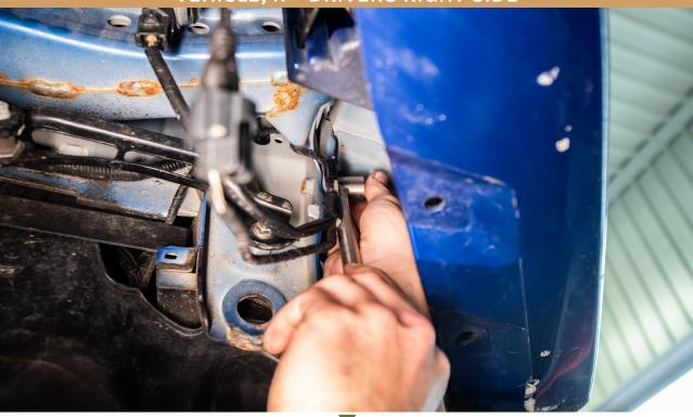
THREAD IN SUPPORT ROD BUT DO NOT TIGHTEN ALL THE WAY
