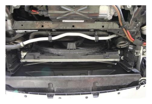
Step 4: Following the same procedure, reinstall CTS Turbo intercooler. Make sure the intercooler tabs line up with plastic guides. Secure intercooler using factory T25 torx screws.
