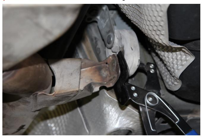
Step 2 - Loosen the clamp from the down pipe and remove factory catback
