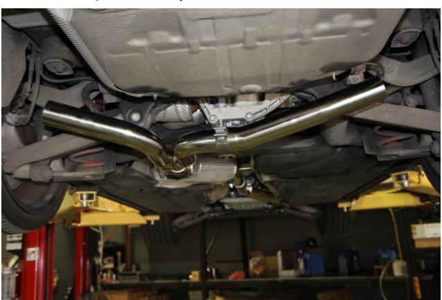
**Step 5 -** Transfer Hanger to the new muffler
