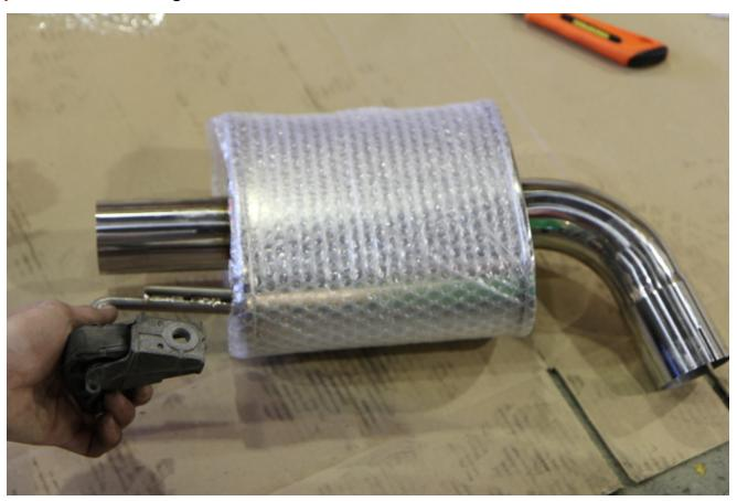
Step 6 - Slip the driver side muffler onto y pipe and attach hanger
