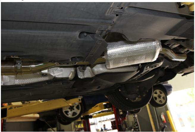
**Step 4** - Install y pipe and passenger pipe **Note:** Leave the clamps loose for adjustment
