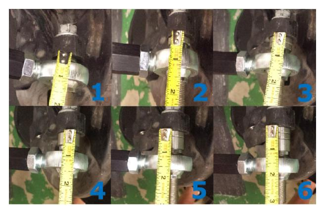
For most installations on stock knuckles, we recommend using 4th setting.
