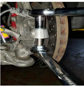
Remove the two 5/8''-18 Jam Nuts, and install the Spacers (3, 4, 5). Install the locking nut on bottom (9). Torque to 80 **ft-lbs**.
