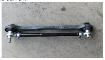
Set SPL Parts Rear Toe Arm next to the OEM arm. Use the bolts through the stock arm to set the SPL Parts Arm to the exact length of the OEM arm ensuring equal thread engagement on both ends. Note: the groove on one side of the arm to indicate the left-hand threaded side.
