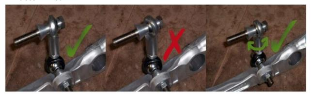
7. Once both sides of the sway bar are attached without any preload induced into the system, tighten down both sides to 30 **ft.-lbs**.
