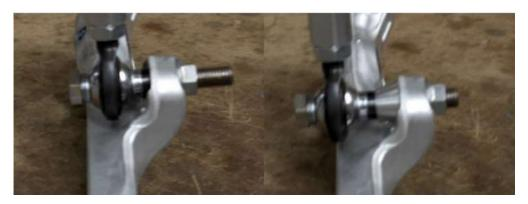
4. Install one end link into the sway bar. As shown in the images on the next page, make sure both rod ends are in the middle of their articulation, and the end link is as close to perpendicular to the ground as possible. When installing the new SPL Parts end links, you should not have to apply any force to the control arm or the sway bar to install the
