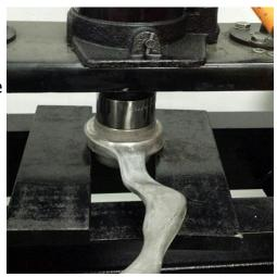
Be sure to have the arm level so the driver/socket can press out the bushing straight to avoid binding. Once square, press out the old bushing. Clean the bore of the arm, and smooth any nicks or burrs. The same socket can then be used to drive in the new bushing. Again, make sure to align the driver and bushing to go in straight and not bind.
