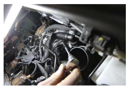
**Step 4:** Install the replacement CTS Turbo diverter valve assembly and tighten the 3x 5mm bolts.
