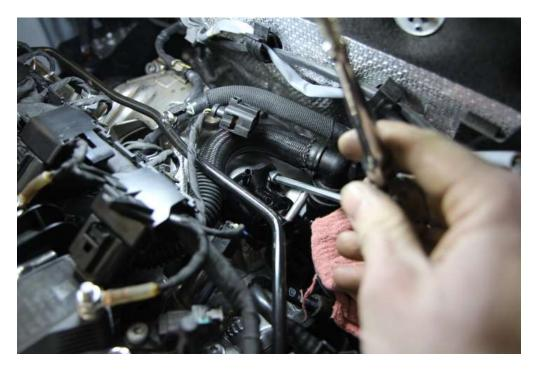
**Step 5**: Note the placement of the T-Connector on the OEM line. See the next step for line routing.
