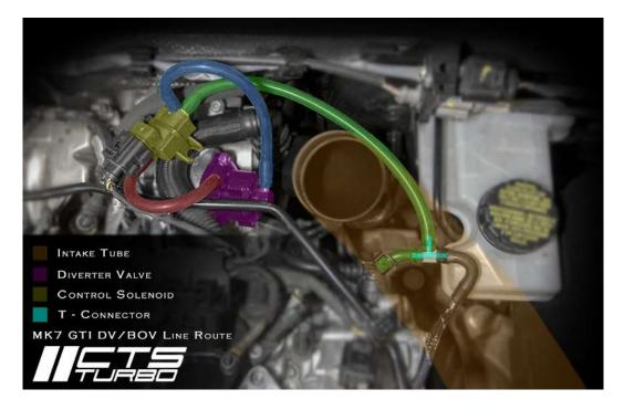
**Step 7:** Reinstall the intake and test drive vehicle. Enjoy your new Diverter or Blow Off Valve.
