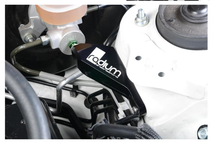
**Completed Installation (strut tower bracing removed for clarity)**
