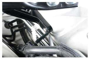
4. Using a 1/2" wrench, unscrew the bolt installed in step 2.
