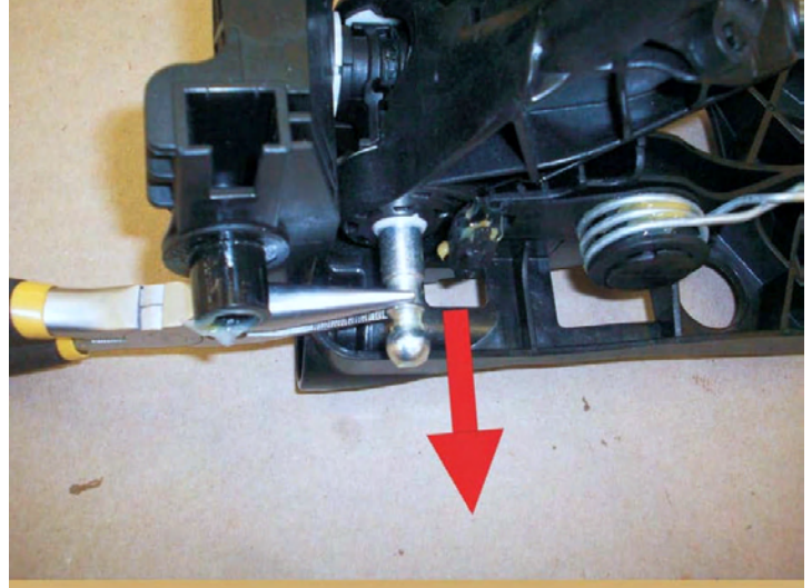
20. Pull the shifter pin out with needle nose pliers.
