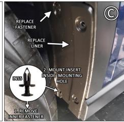
**FIGURE D** Noting placement of INSERT INS5, SPACER.25SP installs in front of INS5, behind mud flap. Use finger to press INSERT head down to prevent spinning while expanding its base.
