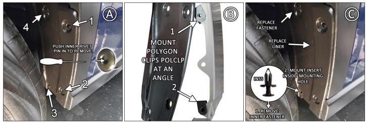
**FIGURE D** Noting placement of INSERT INS5, SPACER .25SP installs in front of INS5, behind mud flap. Use finger to press INSERT head down to prevent spinning while expanding its base.
