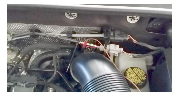
On MK7.5 GTI PP and 245ps Skoda and all cars fitted with the new particulate filter you will find the O2 sensor is different and it has 6 output wires. Connect blue AFR wire to white.
