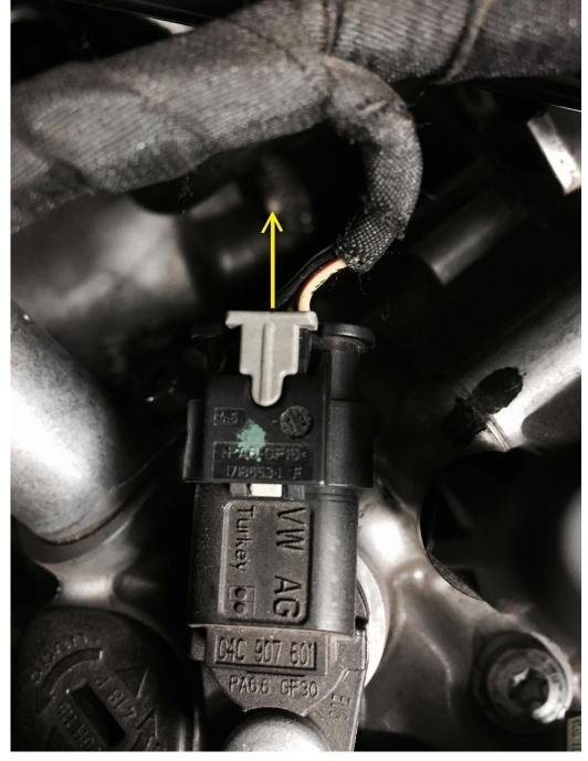
**PLUG B:** The boost sensor plug on the manifold is removed by pushing the grooved tab down on the end of the sensor (yellow square) and pulling the plug towards the back of the car. Plug the removed plug into the male plug on the JB harness and the female plug from the JB harness into the sensor. Once JB plug is put in sensor lock by pushing grey tab towards sensor.
