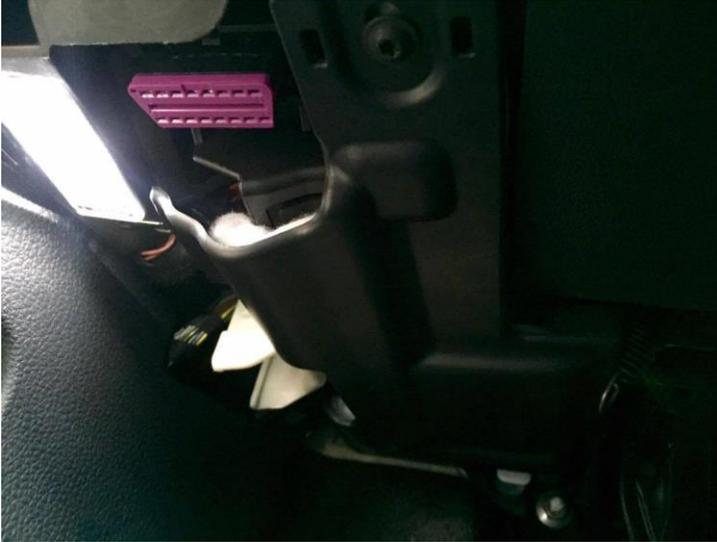
The panel can be removed by removing the hex screws holding it in place.
