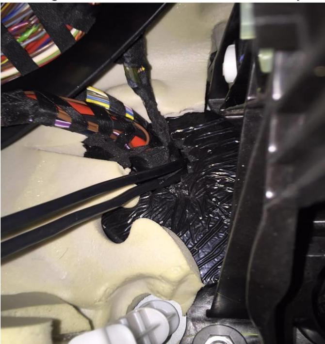
The wire will come out of an area behind the battery and can be run to the JB4 unit and plugged into the Molex plug. It is essential the male and female molex plugs are connected the right way round with no force needed.
