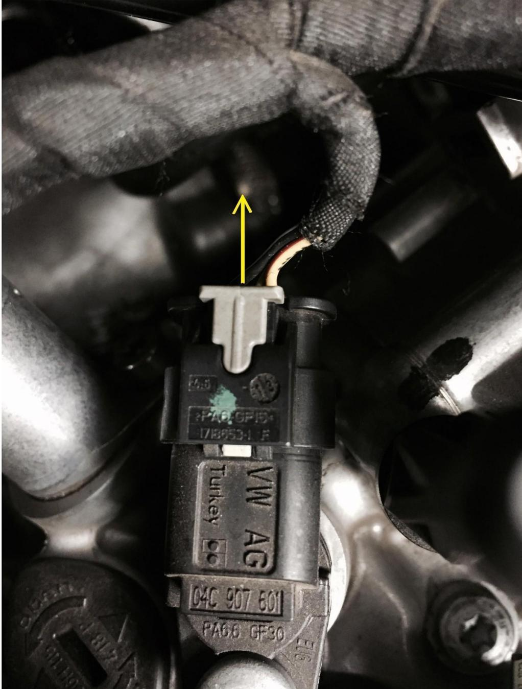
**PLUG B:** The boost sensor plug on the manifold is removed by pushing the grooved tab down on the end of the sensor (yellow square) and pulling the plug towards the back of the car. Plug the removed plug into the male plug on the JB harness and the female plug from the JB harness into the sensor. Once JB plug is put in sensor lock by pushing grey tab towards sensor.
