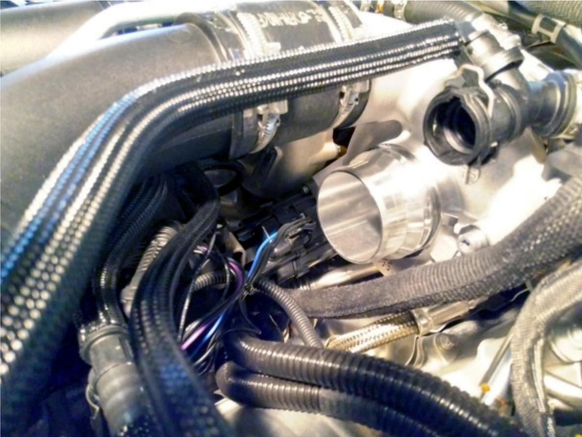
After plugging in the connector slide back in the inlet and reinstall the intake tube.
