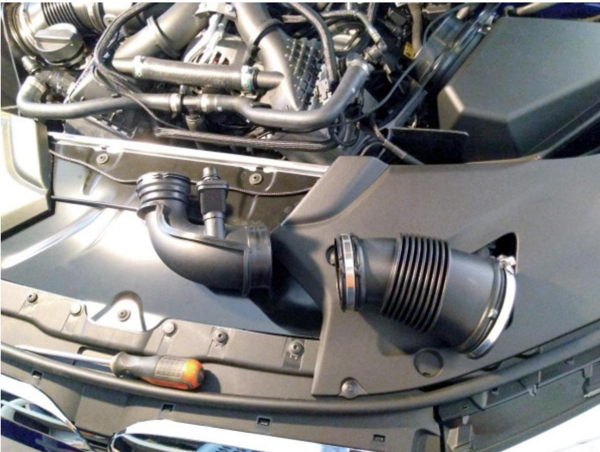
With the inlet removed plug the EWG\_A connector in the same way EWB\_B was connected.
