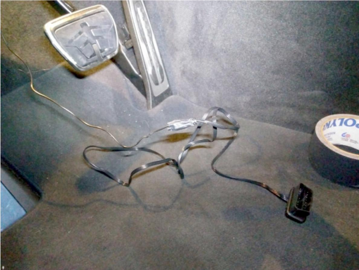
From the engine bay pull the OBDII cable out and plug it in to the matching connection on the JB4 harness.
