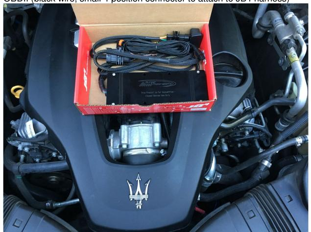
To view the connectors you will have to remove the engine cover. Pull up and it will
