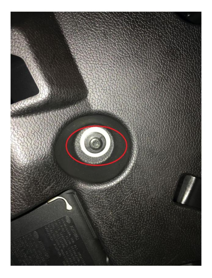
Once you remove the under panel, you will need to route the OBD cable through the fire wall. The best place will be through the steering shaft.
