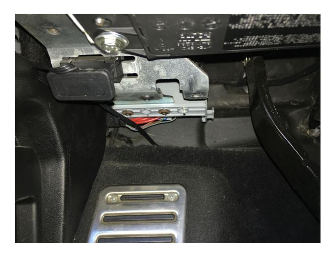
Cable will come through this area where the steering shaft comes through the firewall. You will pull the cable and route it up and over the shock tower towards the front where the Jb4 will sit.
