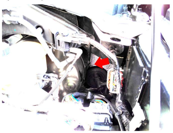
Route the OBDII cable along the firewall tucking it over the brake booster and other factory mounts to keep it from sitting on the engine cover and plug in to the matching JB4 connector.
