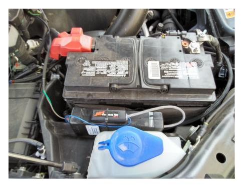
If installing Stage1 installation is complete. If installing a JB4 there is an optional OBDII cable to route under the drivers seat. If not installed the JB4 will act like a Stage1.
