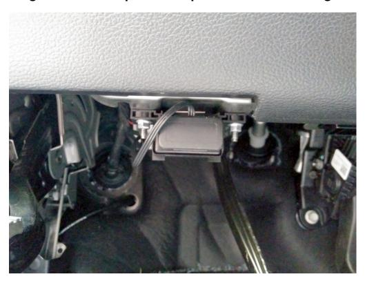
Push out grommet from under dash and pass OBDII wire through to engine bay. After attaching it to the JB4 harness push the grommet back in from the engine bay over the wire you've routed.
