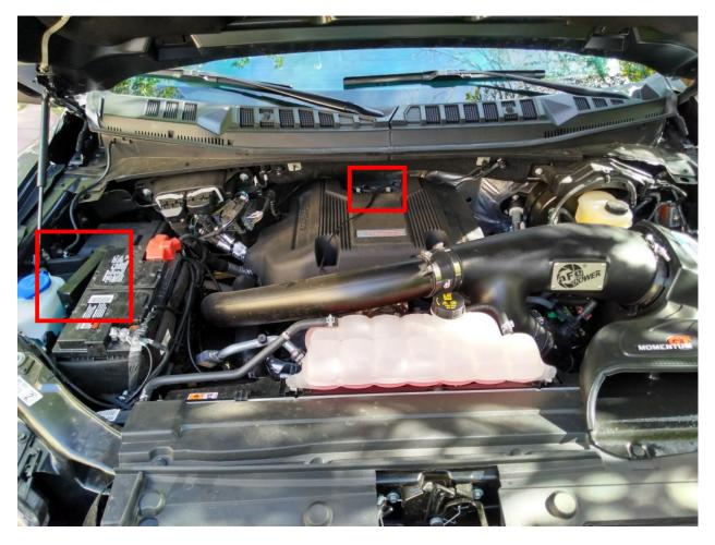
Install box placement shown with optional JB4 Mobile adapter.
