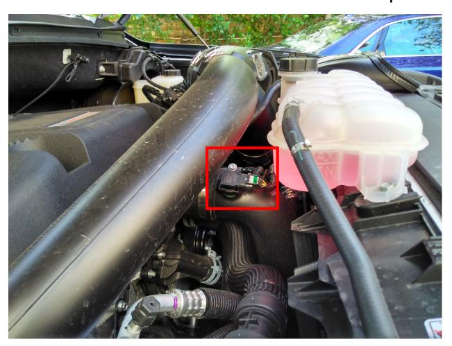
Attach the rainbow connection to the MAP sensor shown below. Finally, route the cables and place the control box next to the battery.
