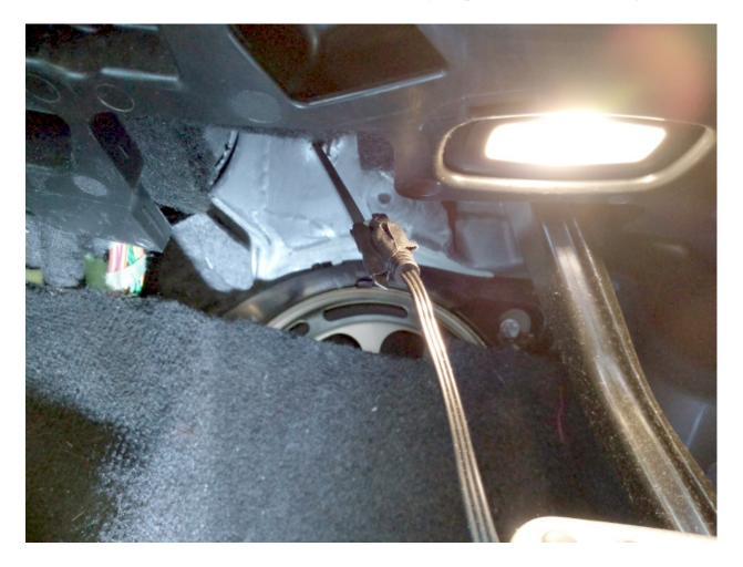
The result will be the OBDII cable passed in to the engine bay which you'll plug in to the JB4 harness.
