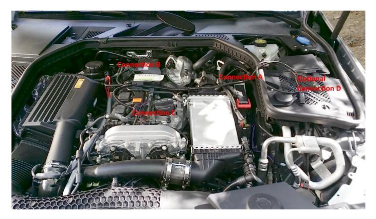
A) Rainbow wire patch, 3 positions Both JB4 & Stage1: Connect to TMAP connection A.
