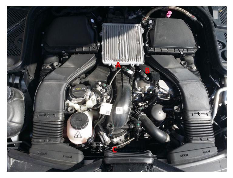
A) Rainbow wire patch, 3 positions Stage1 & JB4: Connect to TMAP connection A.
