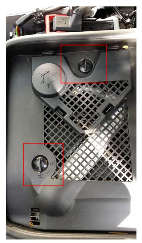
Place the wiring harness with control box attached under the plastic cover behind the brake booster as shown. You can secure the box to the brake booster area with a zip-tie, or simply wedge it between the brake booster, and the engine cover. Care should be taken to ensure the box is not left under the grated area of the engine cover where water could drip in to the control box.
