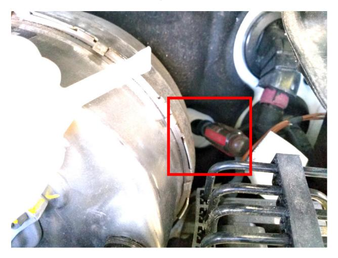
Inside the car under the dash tape the OBDII cable to the screwdriver so when you pull it out the OBDII cable follows. Alternativelty you can just poke the cable through the hole manually.
