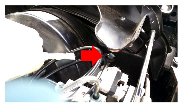
Plug the OBDII wire in to the JB4 green/brown pair connector.
