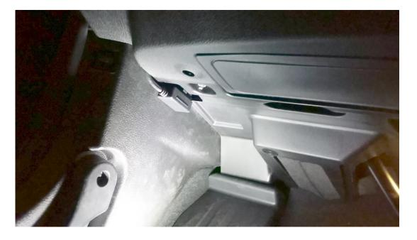
6) Tuck the now fully installed JB4 control box out of the way as shown. The wiring harness should be routed under the rubber cowl seal for a clean fit once the cowl cover is reinstalled. Tuck any extra wire length out of the way taking some care to ensure nothing is too close to the moving mechanical parts of the windshield wiper arm/assembly.
