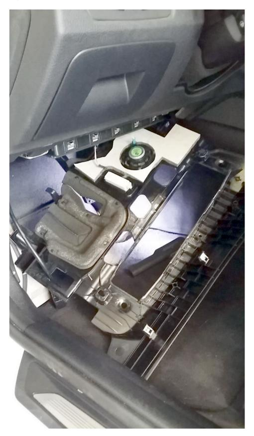
Using a long screwdriver push in on the rubber firewall cap pushing it in to the interior compartment. You'll see it fall down by the pedals and can put it away for safe keeping. Feed the OBDII wire from the interior through the hole to the engine compartment.
