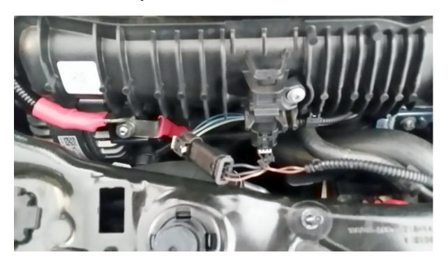
4) Locate the TMAP sensor, unplug it as you did the MAP sensor, connect the JB4 rainbow patch to the sensor, and connect the OEM harness to the JB4 rainbow patch.
