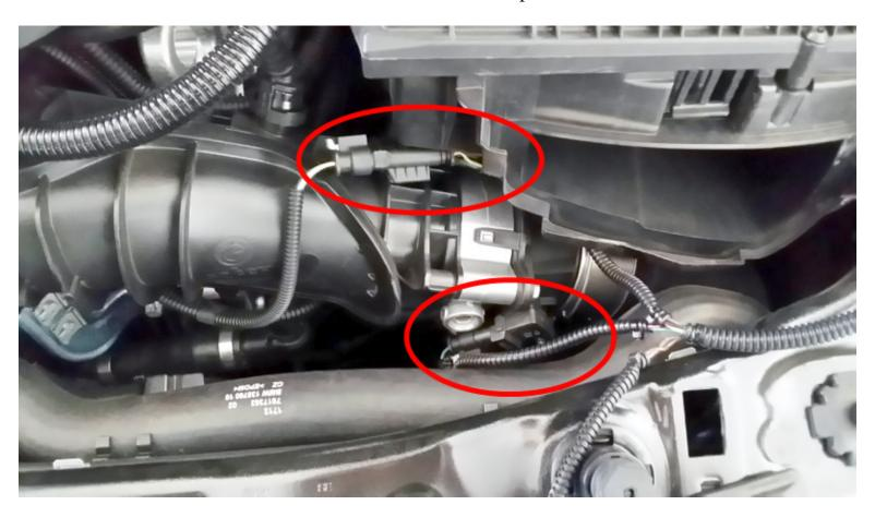
5) Route the harness towards the driver side as shown and reinstall the air duct removed in the first step.
