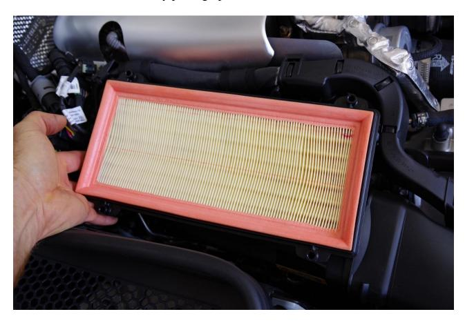
Remove both airboxes, then place a clean rag into each turbocharger inlet to prevent any foreign debris from getting into the turbochargers.
