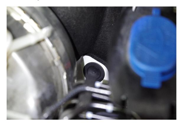
Remove this cover and, using a sharp tool like an awl or utility knife, make an incision into the rubber underneath. A photo of an awl poking through from the engine compartment is shown below.
