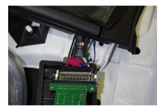
Connect the 9-pin connector to the other end of the JB4 circuit board and secure with the supplied screws. Route the gray wire through the small hole in the JB4 enclosure, and if desired, secure with zip ties as shown.
