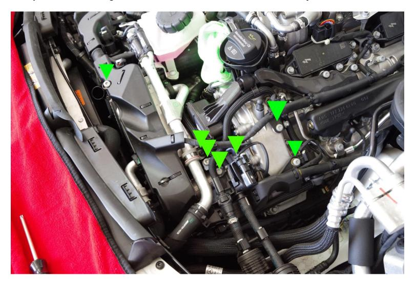
Release the harness from the standoffs at the valve cover as shown if needed for additional clearance.
