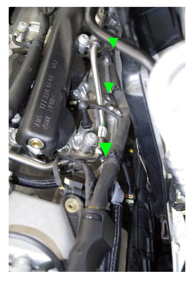
You should now have enough clearance to slightly lift the plastic harness shroud. MAP sensor 1 is shown in the photo below. If you find you do not have sufficient clearance, look for any areas where the shrouding or wiring is taut. Disconnecting additional sensors or fasteners may be required to gain adequate access on some vehicles.
