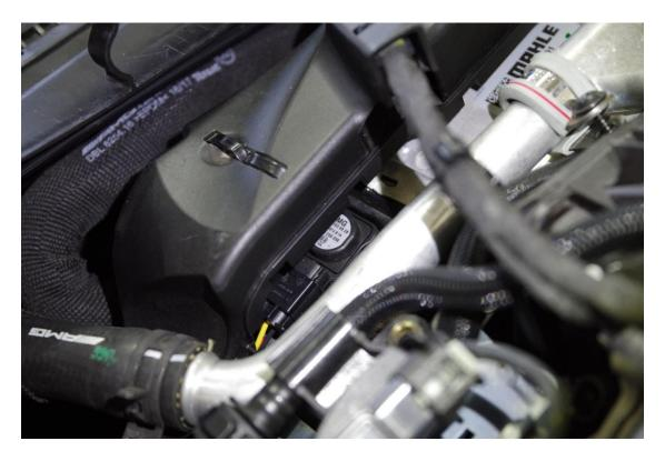
Connect the JB4's male connection to the factory wiring you removed from the sensor as shown.
