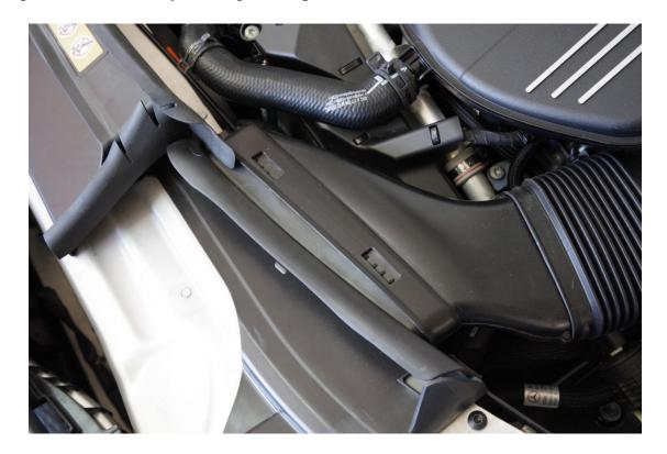
The lower airboxes can be removed by pulling up as shown.
