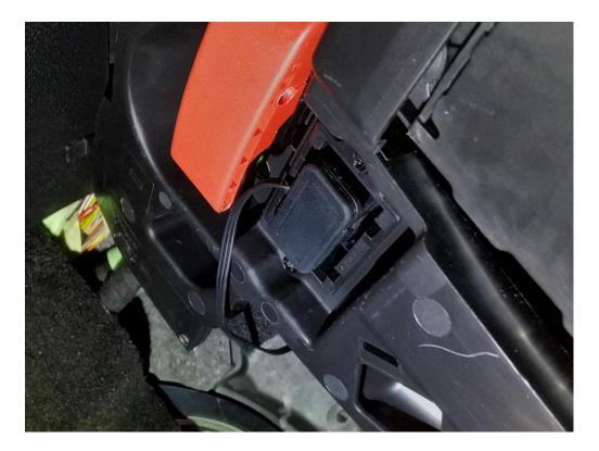
Back in the engine compartment, attach the OBDII cable end to the JB4 harness, noting the orientation of the connection.
