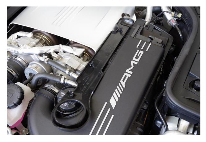
Loosen the four T25 fasteners at the perimeter of each airbox. You do not need to remove these entirely, they will remain captured when loosened.
