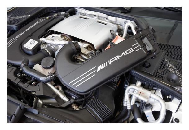
Disconnect the airbox inlets from the trim at the front of the vehicle using a trim tool or screwdriver, or by pressing on the tabs with your fingers. Repeat for both sides.
