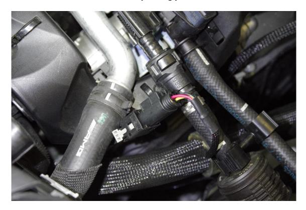
Locate MAP sensor 2. Remove its connection in a similar fashion to MAP sensor 1, by unlocking the tab, then pressing the tab while pulling on the connection to release. Do not pull directly on the wires.
