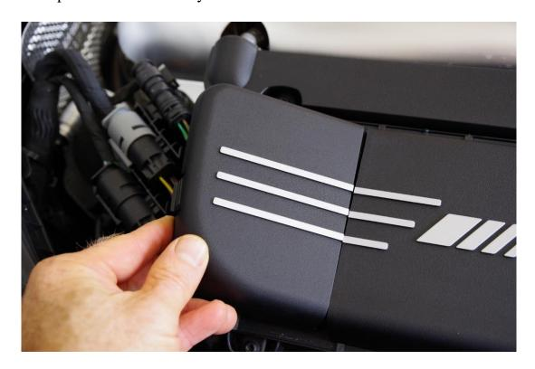
Remove the sensor underneath the cover from the airbox by twisting the sensor while applying pressure. It can be removed when twisted at a specific angle. Repeat at both airboxes.
