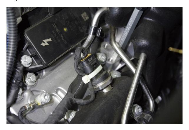
Remove the factory wiring connection in a similar manner to the previous sensors. Place the JB4's orange wire bundle in this location as shown.
