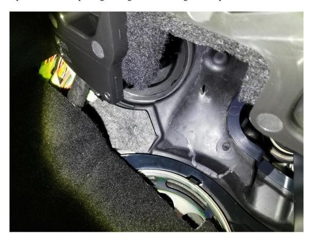
From the driver's footwell, enlarge the opening enough to fit the small end of the OBDII cable through the hole and into the engine compartment. You may want to wrap the end in tape to protect it as you press it through. Attach the OBDII cable to OBDII port as shown.
