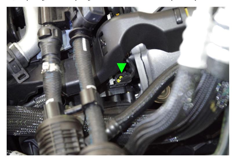
Attach the JB4's brown wire bundle female connection to this sensor, then connect the factory wiring you removed from the sensor to the JB4's brown wire male connection.
