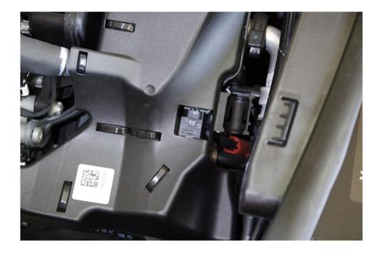
Using a screwdriver or other tool, remove the wiring connection at this location and place the JB4's purple wire connection.
