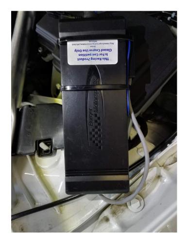
Tuck the JB4's control box into the compartment near the brake booster. Snap the small cover you removed in step 6 back in place carefully over the JB4 harness then and relatch the large shroud over the brake booster area.
