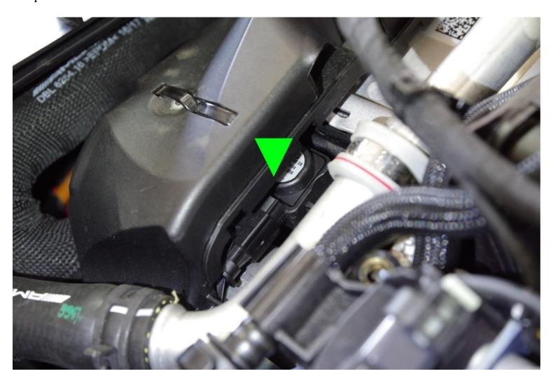
The release clip is found at the front edge of the sensor, toward the front of the vehicle. To release it, you will need to push the tab toward the driver's side of the vehicle first to unlock the tab, then press the tab toward the sensor body while simultaneously putting pressure on the body of the connector. You can use a screwdriver or your fingers for this purpose. Slide the connection off of the sensor.
