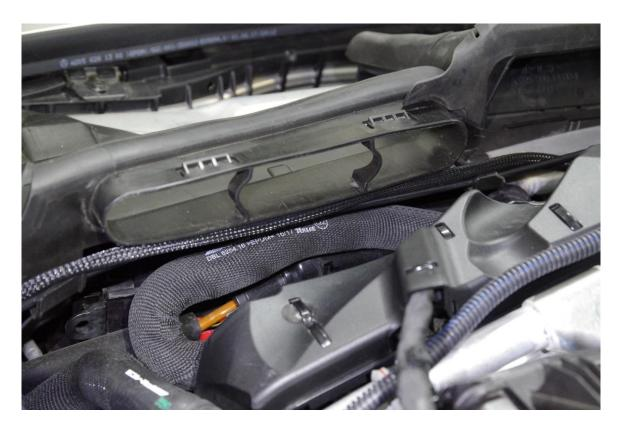
Twist the knob as shown and lift the shroud at the driver's side of the engine compartment (LHD shown).
