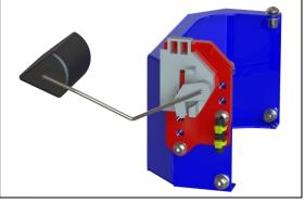
10. <u>Internal Wiring:</u> Find the hanging internal fuel pump connections from the underside of the conductive studs.
