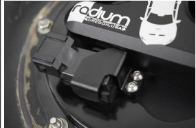
20. External Wiring: Cut off the OEM 5-pin fuel pump control module connector, as shown. Remove some of the tape, and wire loom than strip the insulation on all 5 wires about  $\frac{1}{2}$  back.
