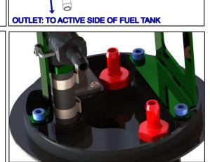
8. Rotate and align the fuel pump(s) concentrically with the cut-outs in the internal pump bracket, as shown in red. Tighten the EFI hose clamps after the alignment is complete. Reinstall the green internal pump bracket. Using the included zip tie, strap the jet pump body to the green bracket. Next, press the filter sock(s) onto each pump inlet and secure with the star washer.
