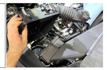
Remove the 2 vent hoses from each valve cover vent port (right side and left side). For EJ25 engines, there are 2 vent ports on each valve over. Do not remove the rear port hoses. Only the frontmost vent ports on the valve covers will be modified.
