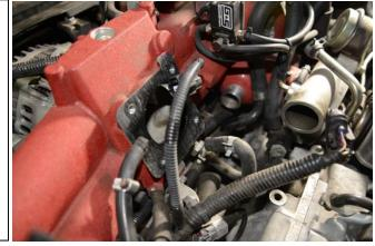
Locate the 3-way TEE underneath the turbo compressor. These will slightly vary depending on the year of the engine.
