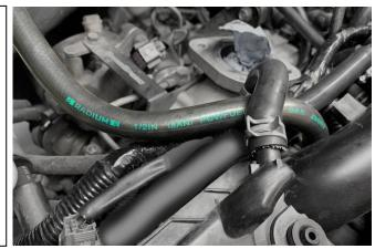
Assemble the 10AN banjo fitting to the AOS-R top port. Make sure the banjo is not upside down and be sure to use a sealing crush washer on each side of the banjo.
