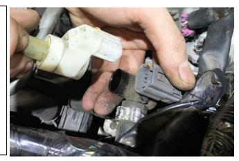
Using a flat head screwdriver, remove the grey wiring connector from the black tube, as shown.
