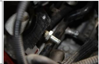
If not already, be sure to remove the small section of rubber hose from the large port on the engine block, as shown in RED.
