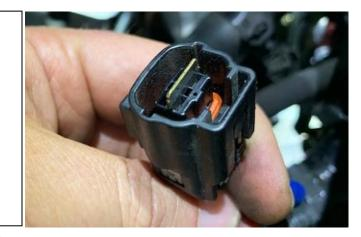
Insulate this wiring junction with electrical tape to prevent accidental shorting.
