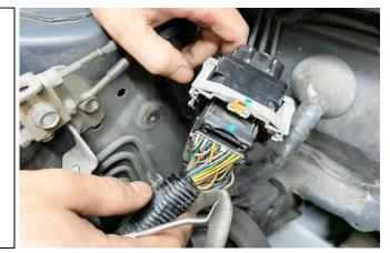
Pully pivot the grey latch. This will disconnect the electrical plug.
