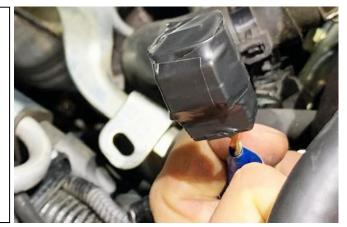
Next, remove this same hose connection from the turbo inlet pipe. This hose will NOT be reused.
